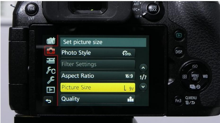
Always keep the largest Picture size (L) and the Quality should be left to the fine JPEG mode which is the double dotted bar until later setups when we will consider the other
