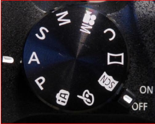
Aperture priority is selected by rotating the top mode control dial to the “A” position. Use the top control wheel to set the aperture or the side control wheel if it has been programmed to F/SS in the custom menu setting for side button.
