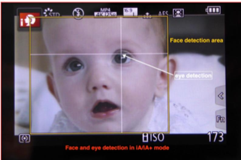
This eye detection mode is automatic and focusses on the nearest eye to the camera. This method cannot be changed.
