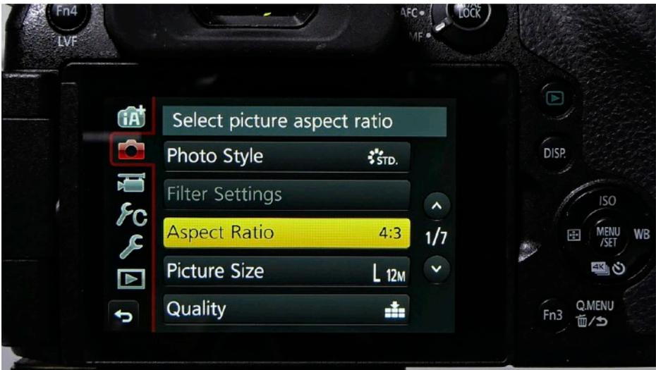
The ASPECT ratio is set from the REC Setup menu (the camera icon tab). This sets the height and width ratio of your image.
