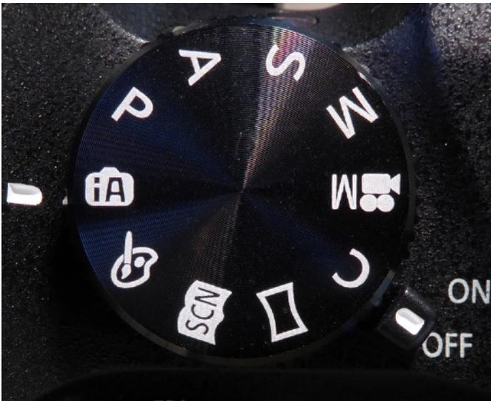
The intelligent auto mode iA is selected by turning the top Mode Control dial so that the iA icon is opposite the white marker on the camera top plate. On the LCD screen you will see the iA icon at the top left hand side of the screen.
