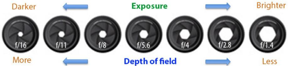
As you can see the aperture size is denoted by a “F” number and this is a mathematical ratio of the diameter of the aperture and the focal length of the lens.
