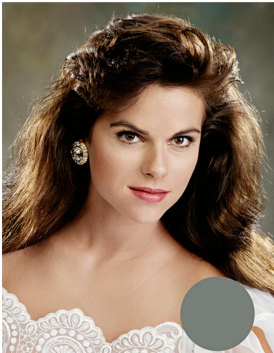
*A typical Kodak “Shirley” with the densitometer measurement patch*
