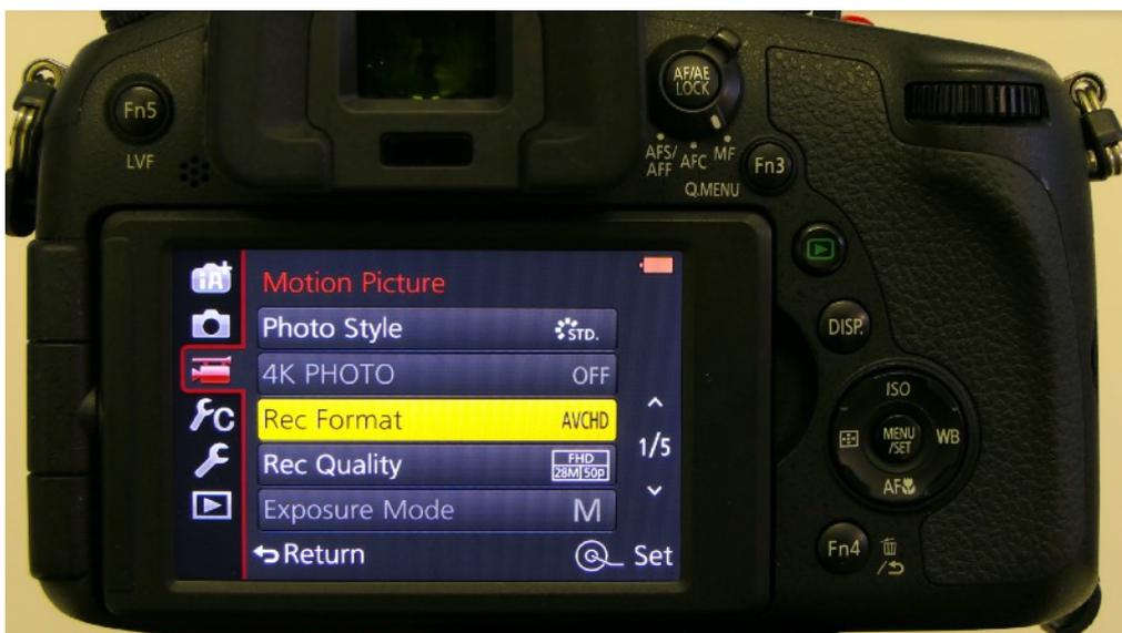
The recording format sets the file output parameters which will include the codec used and the amount of file compression.
