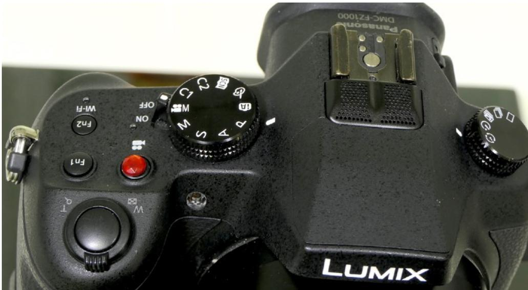
If you want the camera to make most decisions for you then set the camera to be **Intelligent Auto** mode (or the iA+ mode) and the camera will then adjust the exposure as you shoot. It uses its scene detection programming to try and optimise its settings for a type of subject you are trying to record.
