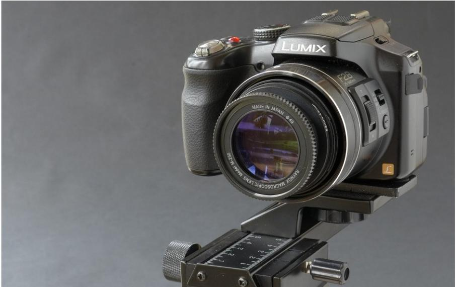
This slide arrangement allows you to set the camera in the manual focus mode and then adjust the camera such that the image is sharp on the back of the LCD. You can use the traversing knob to seesaw about the focus point to ensure you have the exact focus point selected.
